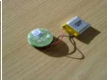
Temperature patch for patient skin temperature monitoring
