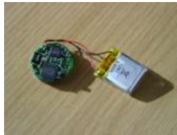
Temperature patch for patient skin temperature monitoring
