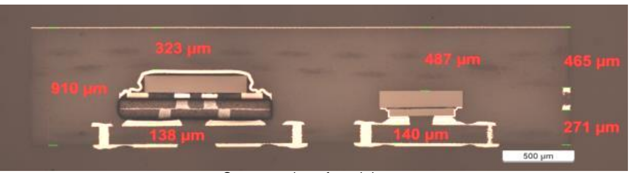
Cross section of module
