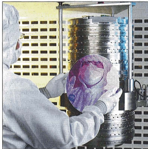
Optical lithography remains the dominant technology for forming transistors on silicon wafers
