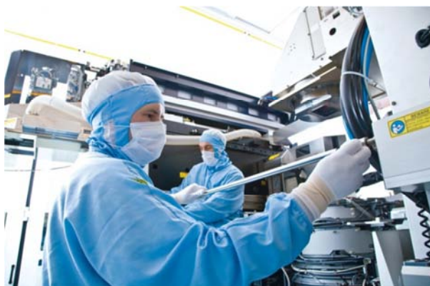
Figure 1. Integration of projection optics in ASML TWINSCAN Wafer Scanner. Source: ASML.
