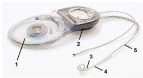
Figure 5.15: The implantable portion of the cochlear implant: (1) Transmitter coil in a silicone sheath; (2): Electronics enclosed in a titanium casing; (3): Electrode with platinum contacts in a silicone array; (4): Cochleostomy site; (5): Silicone cable in the middle-ear/mastoid region. (Photograph from Stöver et al, see [50])
