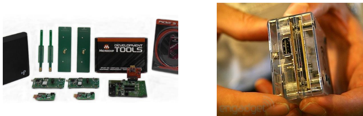
(a) (b) Figure 2.9: State-of-the-art commercial long distance RF harvesting systems: PowerCast [30](a) and Ossia [31](b).
