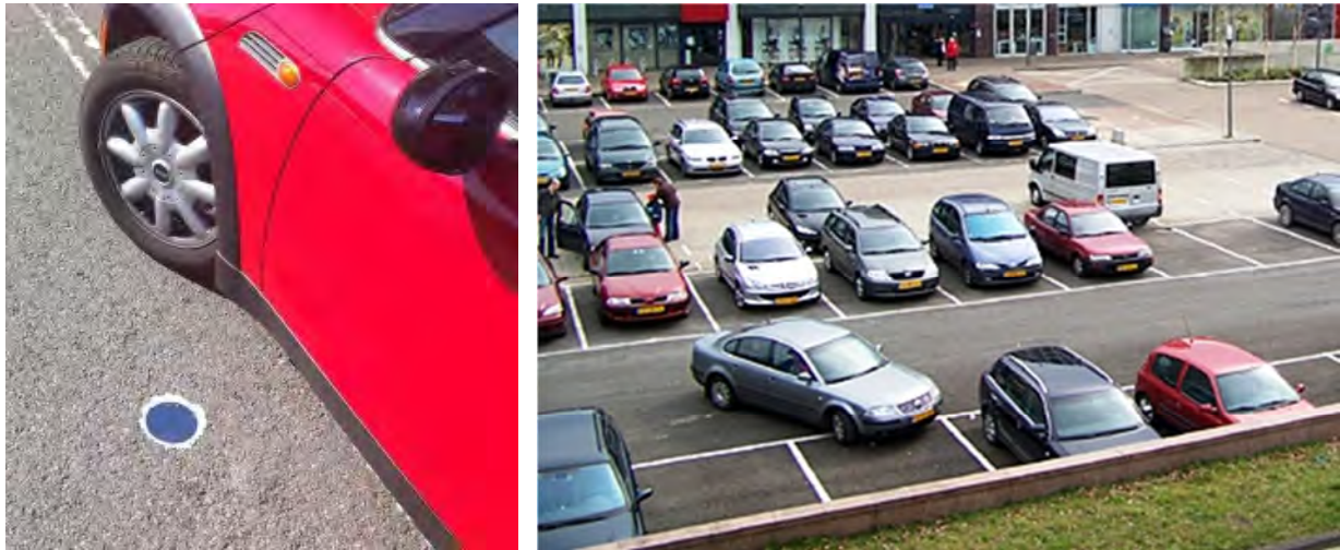
Figure 39: Wireless parking sensors in smart cities
