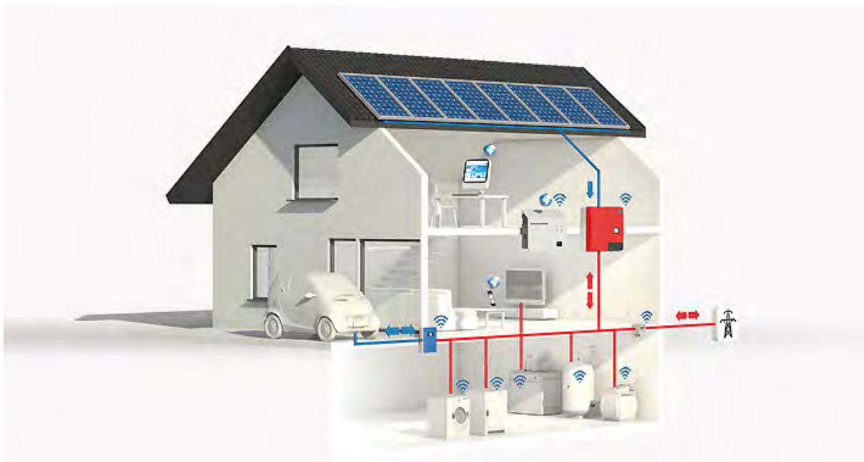
Figure 32: Energy management in buildings means finding the optimum operation strategy using all degrees of freedom that the infrastructure offers: local demand management, local renewable energy harvesting, local energy storage and reception/delivery of energy to the smart grid. 151
